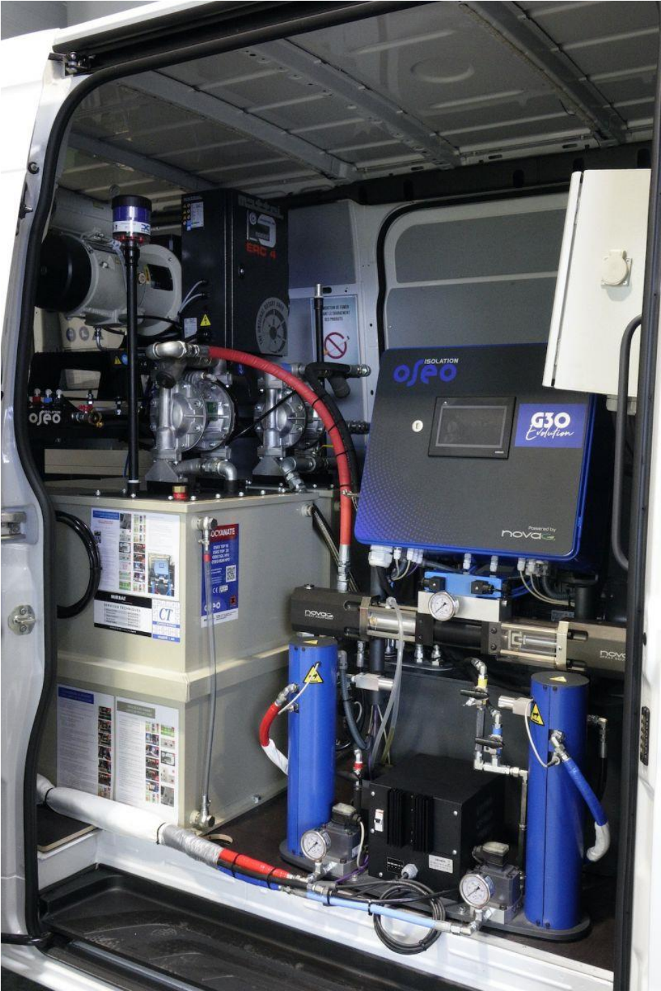
Mirbat has developed trucks equipped for mixing polyurethane components and used by Syneris franchisees and Oseo dealers .
